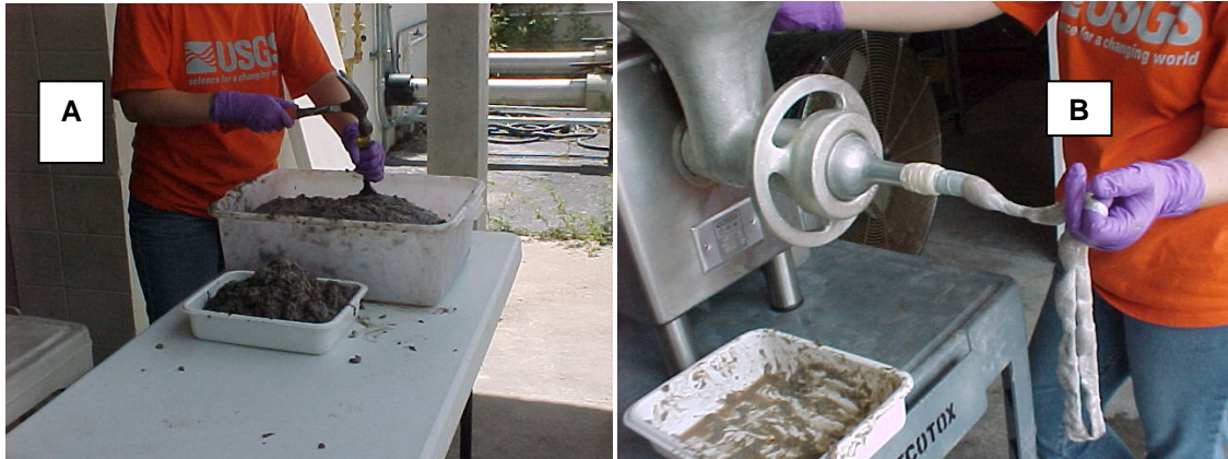
Photographs 3: Production of fish sausages. Fish were initially ground and stored as a single composite of NSRA fish and control fish prior to sausage production and to ensure batch consistency (A). Sausages were produced by re-grinding and extrusion into sheep intestinal casing (B).
